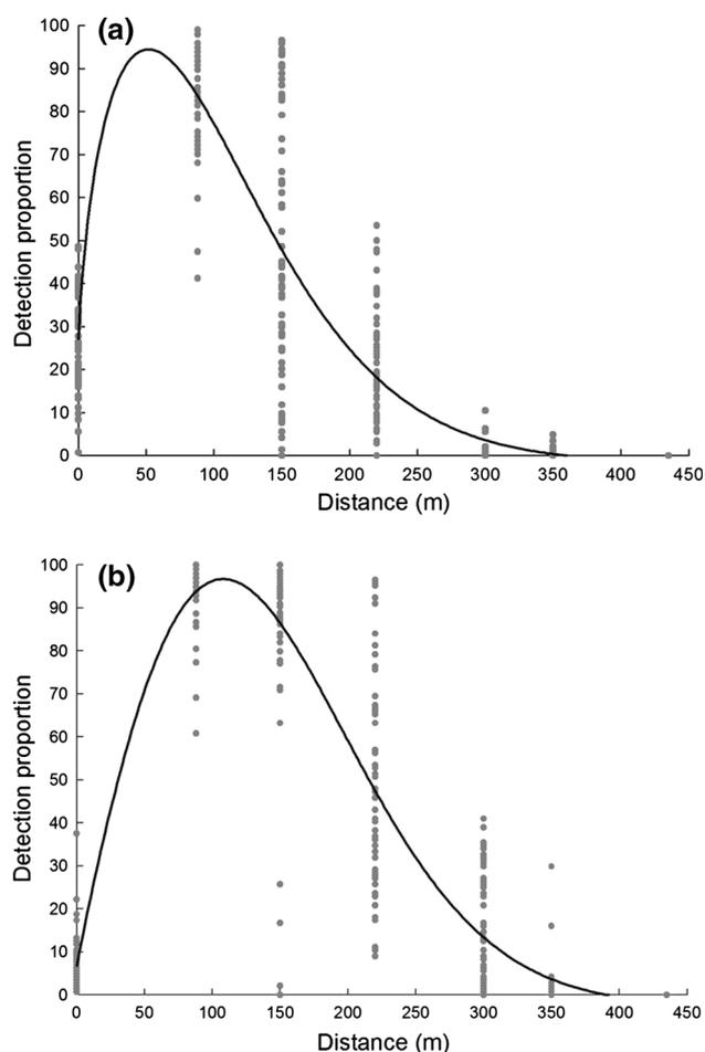
**Fig. 2** Detection range profiles for **a** open-water period (1 August–30 September, 2012) and **b** ice-covered period (1 December 2012–31 January 2013). Effective detection range was defined by the distances at which 60 % of transmissions were recorded
